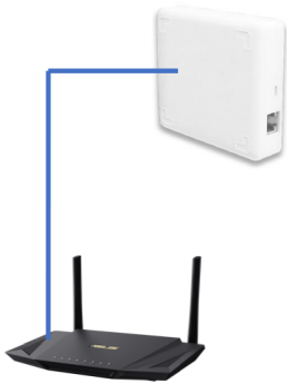
Step 1: Get ready Zigbee Gateway Plug in a Zigbee gateway and connect network cable to the router.
